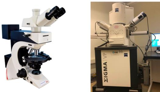
Fig. 2. Polarizing microscope DM2500P used to locate lithic clasts from thin sections (2a); Zeiss Sigma-VP SEM with EDS detector used to analyze lithic clasts (2b).
