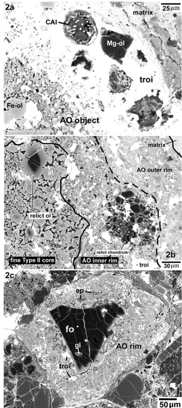
**Fig. 2a-c.** BSE images of (2a) AO-U object Beg-3, showing a micro-CAI, a magnesian olivine (Mg-ol) clast, and other fragments in a troilite-rich periphery; (2b) Beg-6 contains a fine Type II chondrule core surrounded by concentric AO-U rims of two types (coarser inner, finer outer); a relict chondrule is embedded in the inner rim; (2c) NWA-11C contains a fragment of coarse forsterite ('fo',  $\text{Fo}_{99.3-99.4}$ ) grain with glass inclusions, surrounded by an AO-U rim; ep = epoxy.
