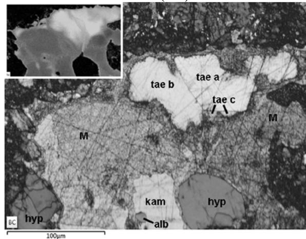
Fig. 2. EBSD band contrast image, with brightness related to crystallinity (brighter = stronger diffraction bands, darker = weaker). Martensite has weaker band contrast than kamacite and taenite. The inset shows a Ni X-ray map. Martensite surrounding taenite is enriched in Ni, forming a diffuse halo. Mineral abbreviations: tae = taenite (tae a, b, c identify different grains), kam = kamacite, ma = martensite, hyp = hypersthene, alb = albitic feldspar, troi = troilite.
