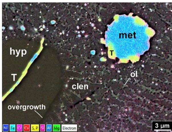
Fig. 3. Element map of representative matrix area. Orthopyroxene (hyp) with troilite (T) vein and overgrowth of clinoenstatite (clen). Met=metal; ol=olivine (light green).
