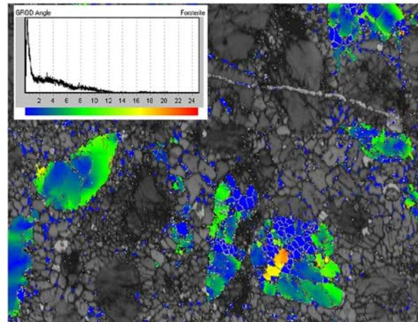
Fig. 4. GROD (grain orientation deviation) angle+band contrast image. Colors indicate the distortion of crystal lattice from a reference value for the grain. Matrix olivines and recrystallized portions of grains have low GROD angle values ( $< 1^\circ$ , blue), whereas clasts are more distorted ( $1\text{-}8^\circ$ , green to orange), with distortion often at their edges.
