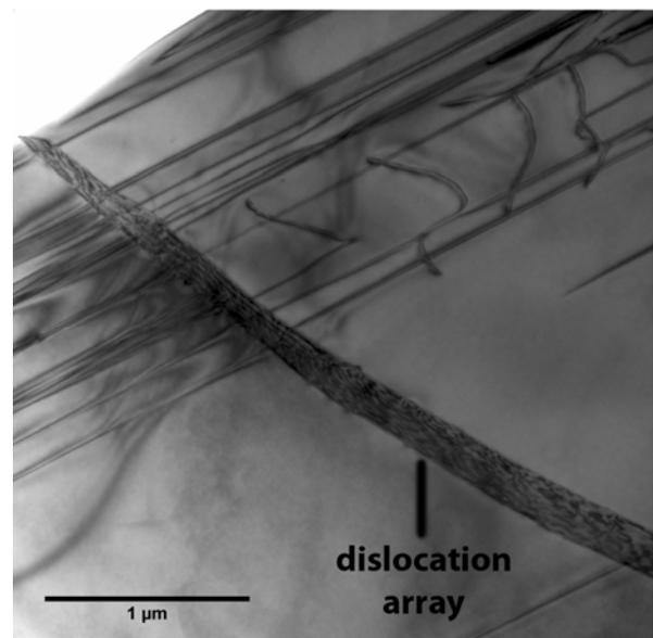
Fig. 2: Bright field image showing dislocations along different slip systems. The straight dislocations jog at the dislocations array, indicating that the array formed after the straight dislocations.
