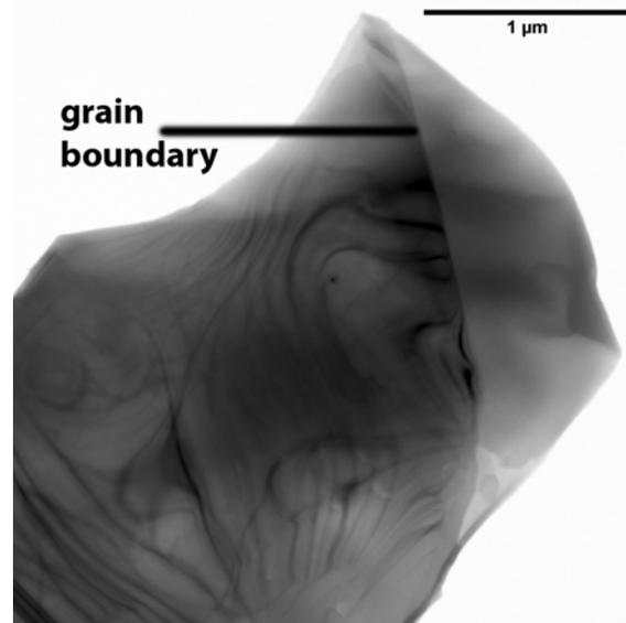
Fig. 1: Bright field image of two olivine grains lacking dislocations. Bend contours and a grain boundary are visible.
