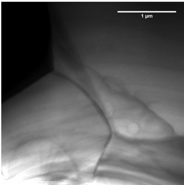
Fig. 4: Conical dark field image showing 120° triple junctions.
