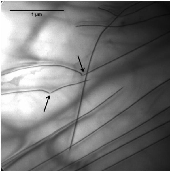
Fig. 3: Bright field image showing two sets of dislocations intersecting each other. Arrows point to dislocation jogs (pinning points) formed at prior dislocation intersections..
