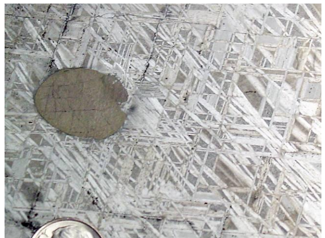
A close-up from a large slice of the Muonionalusta IVA iron donated in April 2010 by Edwin Thompson showing Widmanstätten texture. The large ellipsoid is a sulfide inclusion. A portion of a dime is visible.
