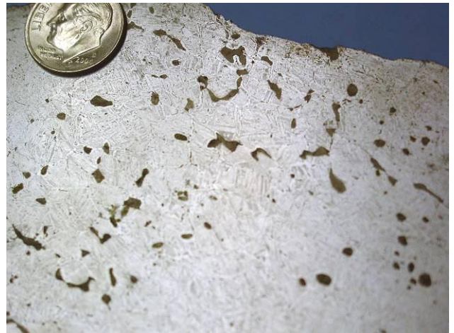
A close-up of the intricate texture of the 2 kg end piece of the Mont Dieu iron donated by Gene and Susan Frederiksen. Dark areas are inclusions of sulfide. A portion of a dime is visible.
