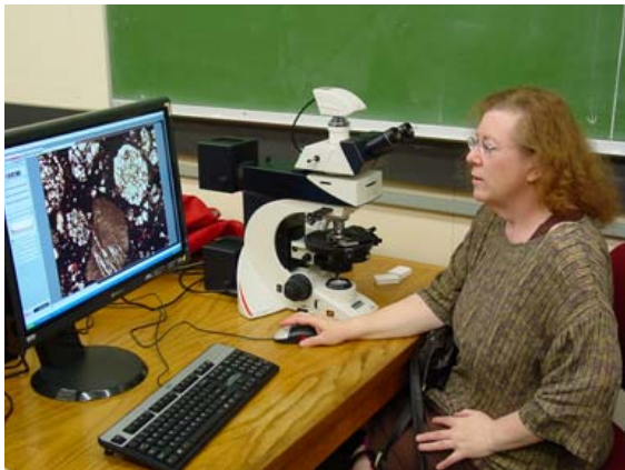
Melinda Hutson uses a petrographic microscope, the basic tool of a meteorite petrologist, to study a meteorite thin section.
