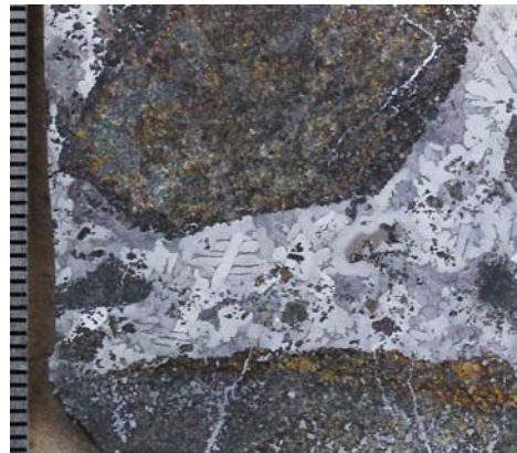
(Above) Backscattered electron image of a relict grain of olivine (dark grain core) in a chondrite (NWA 3127). (Below) reflected light image of an etched silicate bearing iron (Udei Station) containing both silicates (dark) and metal (light). Tick marks at left = 1 mm.
